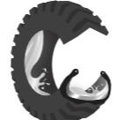
Agri-Seal™ runs around the inside of the tire tread area.
