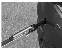
Figure 1: Connecting the vehicles
