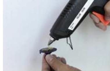
Press the adhesive pad accurately and quickly to the surface of the dent area.
