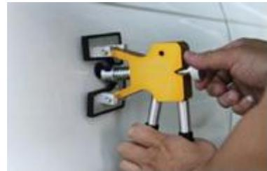
Apply the pulling tool until the dent area is restored.
