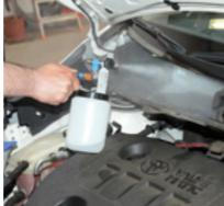
5. Open the bonnet and remove the cabin filter. Clean the pollen filter box if required and disinfect it. Set the ventilation system to level 1 and spray the disinfectant into the interior of the vehicle through the air intake opening of the HVAC system. Feed the agent in until the vehicle interior has become visibly filled with mist. Leave the mist to take effect for approx. 1 minute.
