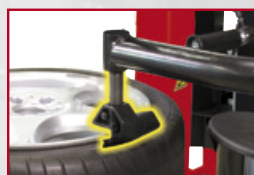
G1000A111 Pressore sagomato WDK WDK bead pressure device WDK- Wulstniederhalter Outil de pression WDK Prensa talón WDK
